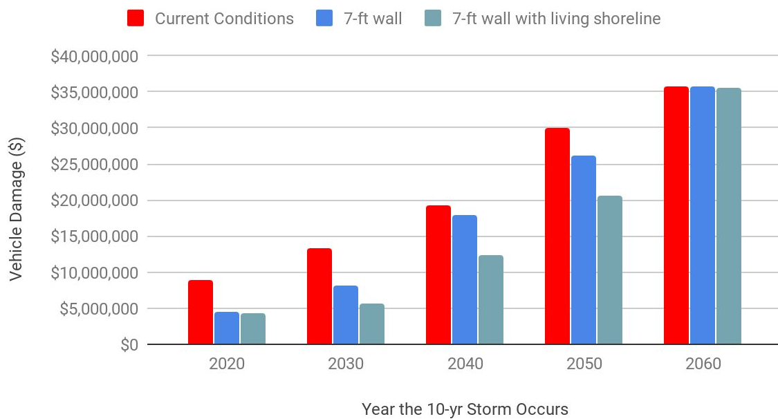
Figure 17: Vehicle Damage from a 10-yr Storm the Year in Which the Storm Occurs
